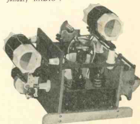
Front view. The neutralizing condenser, a small Cardwell, is mounted on the "upper deck". The Cardwell grid coil tuning condenser is at the right, the plate tuning condenser at the left.
